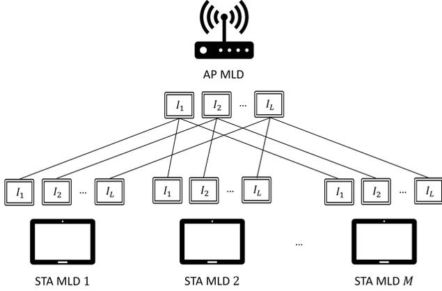
Fig. 1. An illustration of MLO-enabled Wi-Fi network, where  $I_l$  represents the  $l$ th interface and each solid line between interfaces represents a link
