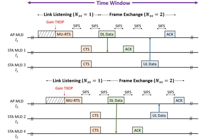
Fig. 2. An example of EMLSR operation in a time window with  $(M, L) = (4, 2)$  and  $\Phi_1 = \{1, 3\}$ ,  $\Phi_2 = \{2, 4\}$ , where  $I_l$  represents the  $l$ th interface and  $N_{ss}$  represents the number of spatial streams in the selected link of an STA MLD in a phase
