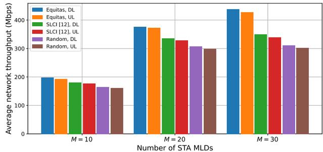
Fig. 3. DL and UL average network throughput achieved by different methods under different numbers of STA MLDs  $M = \{10, 20, 30\}$
