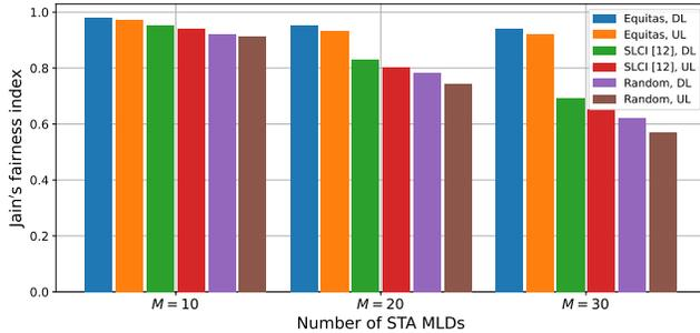
Fig. 4. DL and UL Jain's fairness index achieved by different methods under different numbers of STA MLDs  $M = \{10, 20, 30\}$
