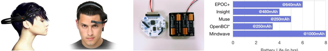
Figure 1. BCI wearable headsets\*: (a) Emotiv EPOC+ , (b) Neurosky Mindwave, (c) OpenBCI System. In (d) we present the advertised battery life and battery capacity of currently popular BCI wearables in the consumer market. OpenBCI system is also our experimental testbed where we implement the wake-up command detection and evaluate the system performance. \* Images for EPOC+ and Mindwave headsets are obtained from <https://www.emotiv.com/epoc/>, and <https://store.neurosky.com/> respectively.
