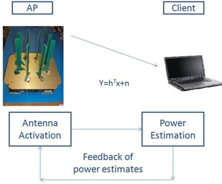
**Figure 1: Beamforming AP and client. The Beamforming procedure is highlighted.**
