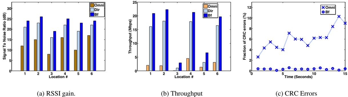
Figure 3: Beamforming improves link quality
