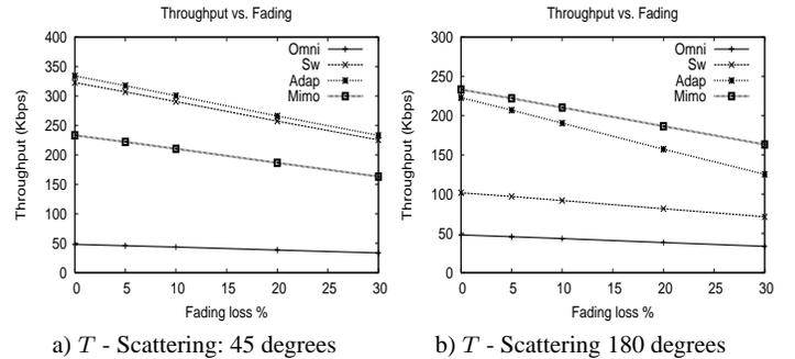
Figure 6. Scattering and Fading
