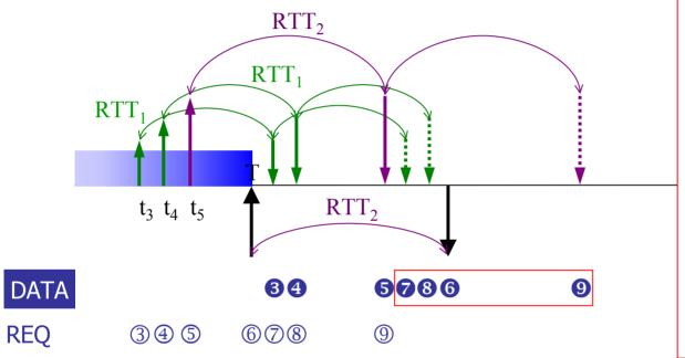
The **binding** data structure maintains the mapping between the R<sup>2</sup>CP sequence number and the RCP sequence number (along with the pipe identifier)
